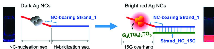
Figure 10. Schematic diagram of red fluorescence enhancement of DNA–Ag NCs through proximity with a G-rich overhang, 3′-G 4 (TG 4 ) 2 TG 3 -5′, caused by DNA hybridization. Photograph of the resulting emission under UV (366 nm) irradiation. Reprinted with permission from reference (158). Copyright 2010 American Chemical Society.
