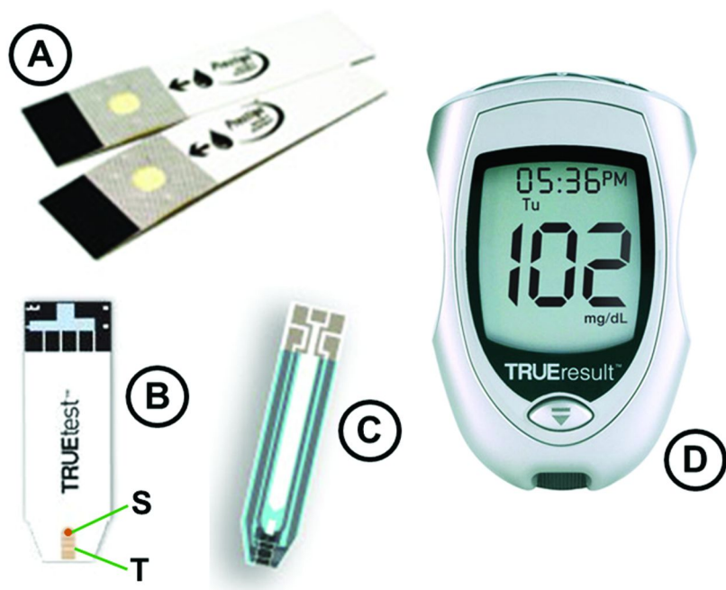
Figure 3. Portable glucose tester (D), manufactured by Nipro Diagnostics, Inc. (Ft. Lauderdale, FL, U.S.A.), and sensor strips (A)-(C). The newer strips (B)-(C) require only 0.5 \mu\text{L} of blood and feature patented quad-electrode design. The sample tip T is 1 \times 3 \text{ mm}^2 and the sensor S itself is 100 \mu\text{m} in diameter. (Reprinted with permission from Ref. (43). Copyright 2012 Nipro Diagnostics, Inc.)
